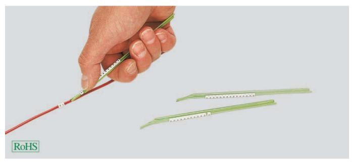
**SR assembly rods**Simple handling afforded by marking rods characterise these marking rings. The nozzle-shaped marking rod is forced onto the line and the snap-on sleeve pushed with the thumb.
