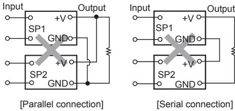
✘ The power supply should not be used in serial and parallel connection in any case. Please use it individually always.
