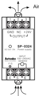
• When installing two or more power supplies side by side, please keep the interval at least 10mm so that the heat is dissipated effectively.
