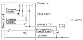
XThere is no short-circuit protection in analog voltage output. Do not connect this output to power supply or capacitive load directly.
