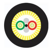
**Cable structure** Core type: Composite buffered GRP support element Strain relief elements: Aramide Type of armouring: Glass yarns Outer sheath material: PE Outer sheath colour: Black
